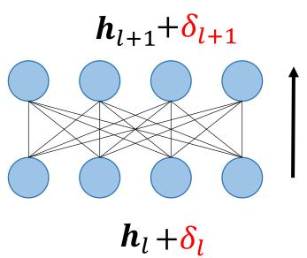
$\|\delta_{l+1}\| < \|diag(h_{l+1} \circ (1 - h_{l+1}))W_l^T\| \|\delta_l\|$
