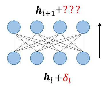
• Forward propagation:  $h_{l+1} = \sigma(W_l h_l) = f(h_l)$
